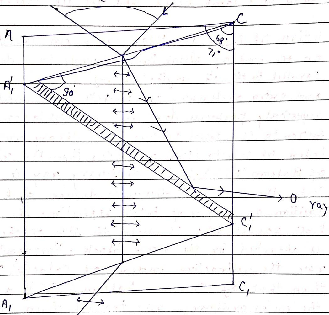
The construction of Nicol consists essentially of rhombic section of calcite crystal whose length is about three times its breadth. The principal section  $ACC'A'$  is parallelogram, whose angles are  $71^\circ$  and  $109^\circ$ . The two end faces of the rhomb are cut down so that the original principal section  $ACC'A'$  of it is now reduced to  $A'C'C'A'$  and its angle reduces to  $68^\circ$ . The crystal is so obtained to cut into two portions by a plane  $A'C'$  perpendicular
